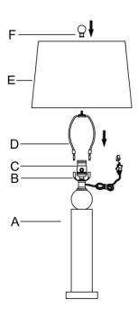
Step 1 Insert the Harp (D) into the Saddle (B). Put the shade(E) on the Harp(D), then tighten the Finial (F)into the Harp (D)
