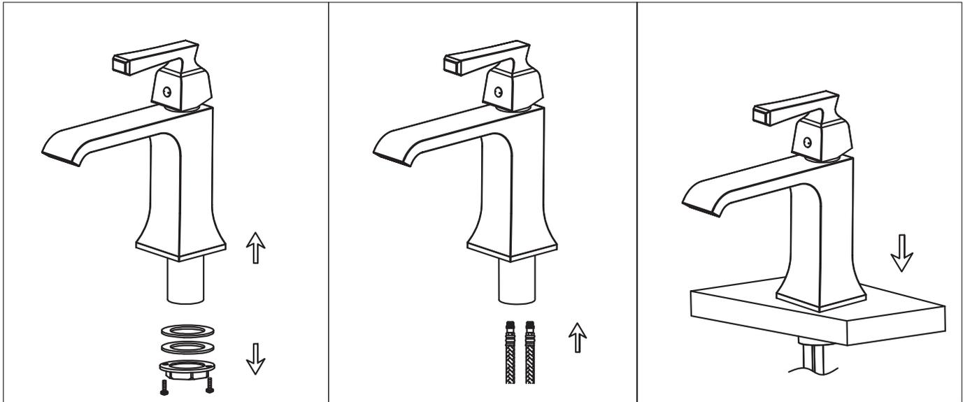
1. Remove the rubber washer, metal washer and locking nut from the faucet.
