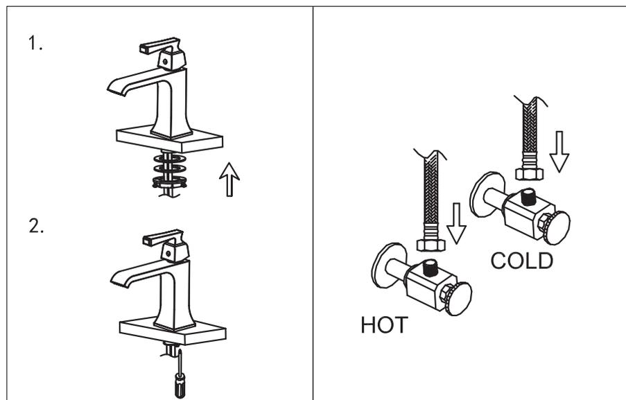
4. Re-install the rubber washer followed by the metal washer and lock-nut. Hand tighten then tighten further using a screw driver to tighten lock-nut screws.
