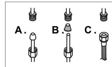
Connect to water supply lines with either:
