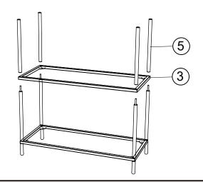
1.Place final frame 3 onto unit and screw ball ends 2 into short poles 5.
