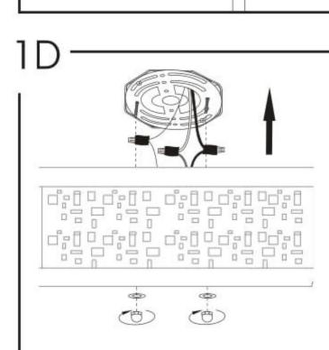
Lining up threads on mounting plate with holes in fixture pan, attach fixture to junction box using cap nuts. Be sure to carefully tuck wires into pan while attaching.
