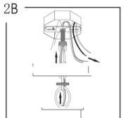
Slip screw collar ring and canopy onto chain, and hang fixture onto screw collar using an open link of chain.
