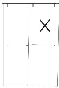
If the glass is in a slanting position after installation, it could be adjusted by the adjusting key, to make sure the glass is to be vertical.
