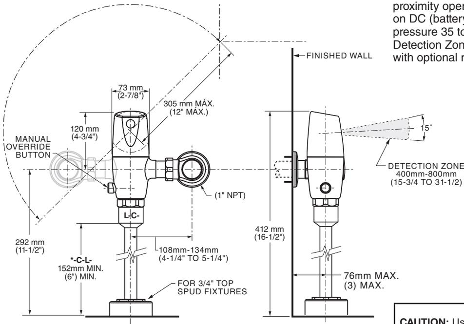
\*Note: The Critical Line (-C-L-) on Vacuum Breaker must typically be 6" (152mm) above fixture. Consult Codes for details.
