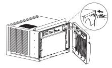
Attach the front grille to the cabinet by inserting the tabs on the grille into the slots on the front top of the cabinet. Push the grille in until it snaps into place.
