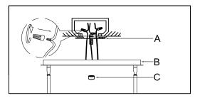
Step.3: Wire fixture to wires in outlet box. Bare wire is Ground wire. Install fixture to mounting bracket using finial (C).
