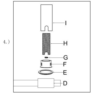
Step.4: Put the round glasses (E) into the cups (D). Put the bulbs (G) onto the sockets which inside the cups (D).
