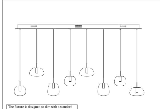
The fixture is designed to dim with a standard Triac forward phase dimmer. Dimming levels will vary by dimmer.
