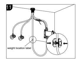
Install the counterweight on the pulldown hose at the marked position. It should be placed on the hose, and secure it with a screwdriver.
