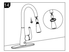
Attach and secure the spray head onto the pulldown hose. Turn on the faucet handle. Wave your hand over the sensor at the base of the faucet. Check for leaks.
