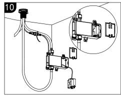
Remove the battery pack cover on control box and take out the battery pack; insert 4 AA batteries (not included). Put the battery pack back in the control box and replace the cover firmly. The batteries should be changed when the sensor flashes a red light. Rechargable batteries can be used.
