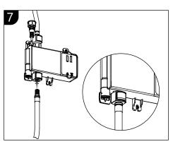
Attach the black nylon braided hose to the adapter at the bottom of the control box until it clicks in place.
