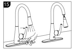
Pull out the spray head. The infrared sensor begins to work when the spray head is pulled out. Slide the hand shower back in and the water will turn off. We reccomend turning the faucet off when it will not be used for an extended length of time.
