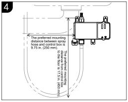
The dimension shown in the figure is a preferred mounting distance for the control box. The distance can be adjusted to better fit your space as required-.
