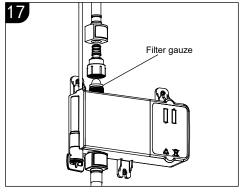
If the water flow rate is lower than normal, there may be built up on the filter screen. Shut off the water valves and remove the outlet hose from the control box. Unscrew the plastic outlet adapter from the control box. Take out the filter screen and clean it. Reassemble the outlet hose connector. Attach the inlet hose to the adapter until it snaps in place.
