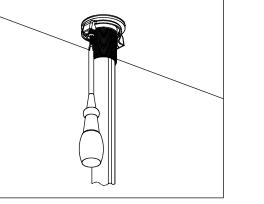
Use a screwdriver to thread the 2 screws tight against the metal washer. Do not over tighten.
