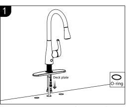
For 1-hole sink installation, insert the O-ring onto the faucet base, over the cable, hoses and the shank onto the faucet bottom, and then mount the faucet on the sink. For 3-hole installation, insert the deck plate over the cable and hoses against the faucet base, aligning the handle so the sensor tab is in front of the sink, and the base aligned across the holes.
