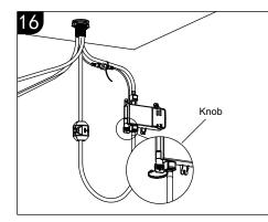
For manual operation, turn the knob beneath the control box counter-clockwise to the end (as shown in figure 16). The sensor will be disabled and the faucet will be activated by the handle only.
