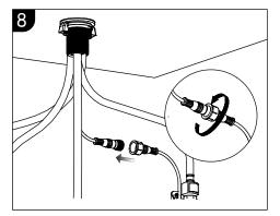
Connect the sensor cables and hand tighten them firmly. NOTE: Sensor is, "Keyed," and installs only one way.
