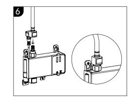
Attach the outlet hose to the adapter on top of the control box with the, "Quick-connection," until the connection clicks.
