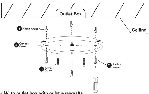
Attach canopy cover (A) to outlet box with oulet screws (D). Screw anchor screws (C) into plastic anchors (B) to secure canopy cover (A).
