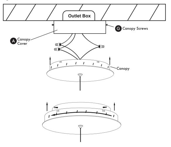
Attach canopy to canopy cover (A). Twist canopy to lock fixture in place. Secure canopy with canopy screws (G).
