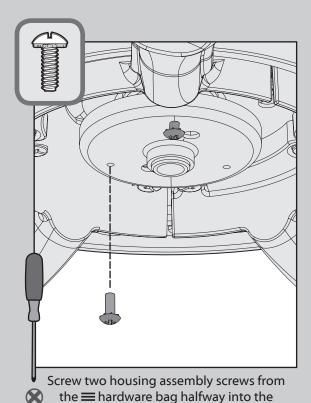
motor housing. It does not matter which
