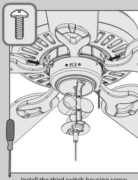
Install the third switch housing screw.
