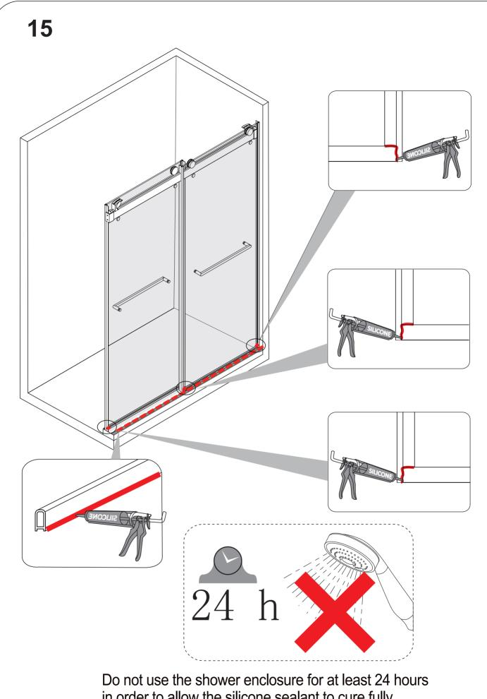
in order to allow the silicone sealant to cure fully.
