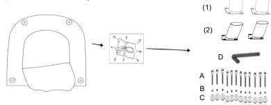
Step 2 : Using bolts (A), lock washers (B), flat washers (C) to connect legs (1) or (2) to chair (3). Tighten bolts (A) with Allen Key (D). Repeat this step for the other three legs.
