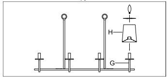
Step8. Place the shade (H) on the socket. 9. Install 8 max 60W E12 bulbs into socket.
