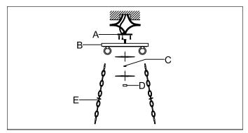
Step2. Remove mounting bracket from fixture and install to electrical box.
