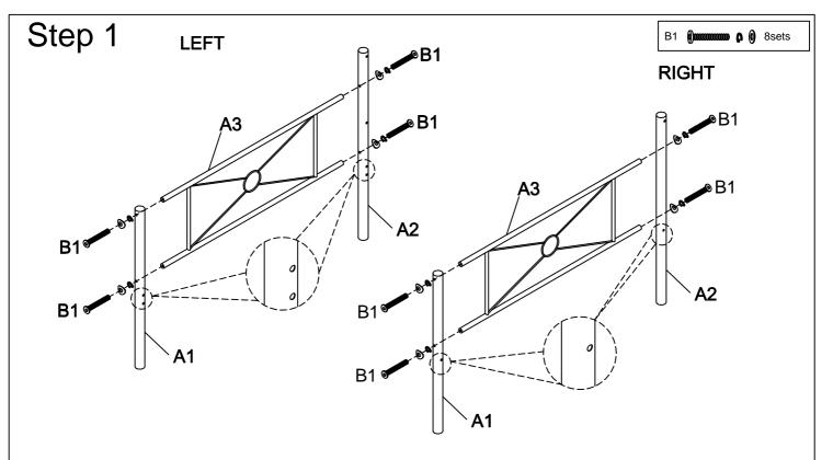
Assemble Side Frames A3 to Front Legs A1 & Rear Legs A2 using Bolts B1 with spring washers and flat washers. (NO TE: Please do not tighten Bolts B1 until Step 5.)
