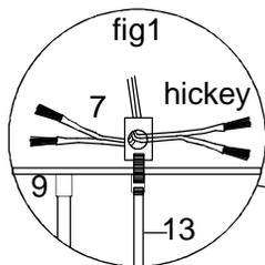
Step8-Lace fixture Main electric cord, ground wire and safety cable through chain every 3 or 4 links. Release bobèche and canopy by unscrewing collar loop ring and pass wire to reach inside of outlet box.
