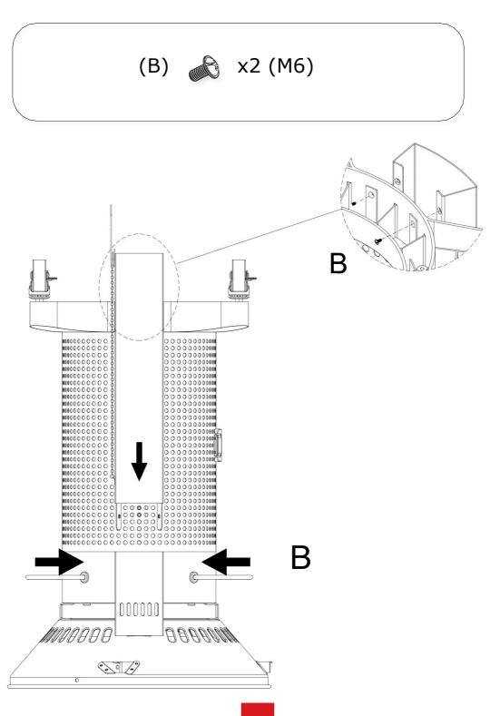
Install front panel: insert bottom hinge first, then use your finger to depress top spring-hinge and release once aligned into position.
