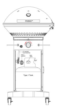
The Professional by Fuego grill is orificed for use with LP gas and comes equipped with a high capacity hose and regulator assembly for connection to a standard 20lb. LP cylinder (Type 1). The LP tank is not included. LP hose and fittings are included. Operating pressure: 11" W.C.
