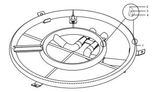
The factory burners have been set for the correct air and gas mixture. The correct flame pattern is shown in the figure to the left.
