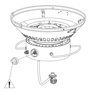
Insert the AA battery into the battery pack with the  $+\$ end facing the battery pack cap.
