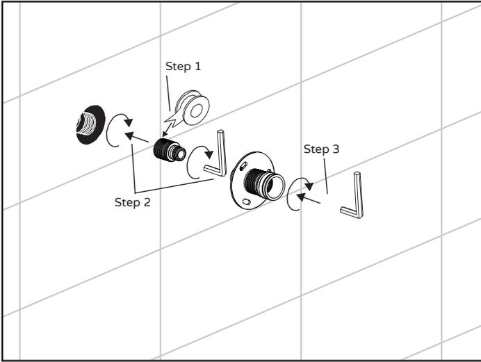
[Step 1] Apply a generous amount of PTFE (plumber's) tape to end of end of inlet fitting (9).
