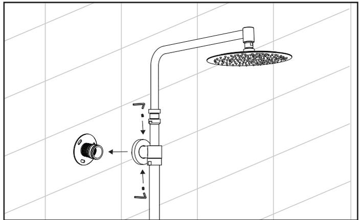
Secure shower bar to fitting and secure with set screws.
