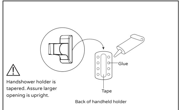
Apply glue to the handshower holder (14) as indicated and add tape (included) to secure onto wall. Let it cure for 48 hours for complete result. Handshower holder is tapered. Assure larger opening is upright.
