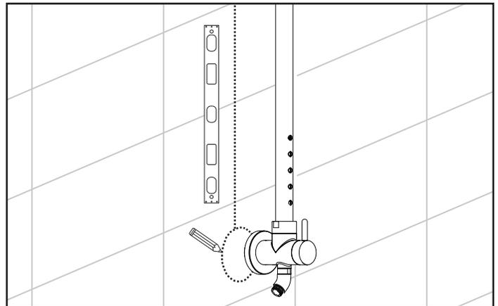
Use level to assure shower pipe is straight and mark lower diverter mount location.
