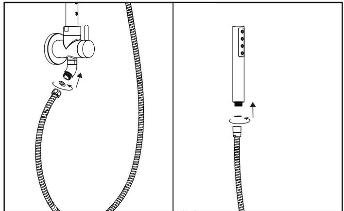
Insert washer (2) into the hex end of the hand shower hose (15). Attach hose to hand shower (13) outlet located on the bottom of the diverter (16).
