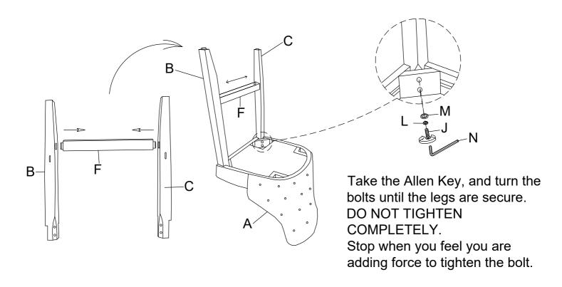
First, attach the Rear Stretcher (I) to the Left Rear Leg (D) & Right Rear Leg (E). Then attach them to the Chair Body (A) using Bolt (K), Lock Washer (L), Flat Washer (M) in both holes of Chair Body (A). Turn the Allen Key (N) in Bolt (K). But not too tight. Second, attach Right Stretcher (H) to Front Right Leg (C) & Right Rear Leg (E), and attach Left Stretcher (G) to Front Left Leg (B) & Left Rear Leg (D) as below shown.
