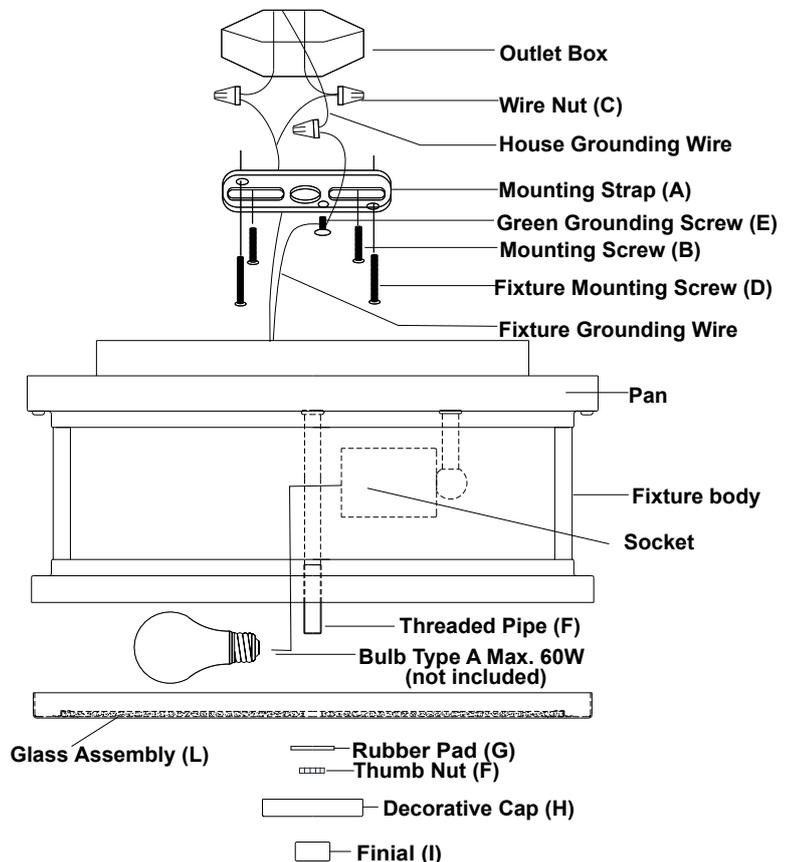
1. Attach the two fixture mounting screws to the mounting strap, and screw in 2 to 3 turns.
