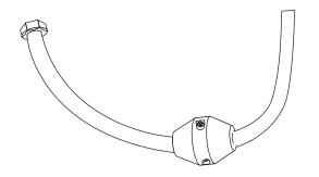
6. Attach your main water lines to the copper water supply posts on the faucet. Ensure that you are connecting the hot and cold in accordance with the labels on the supply posts. Apply a bit of thread sealant or plumber's tape to the threads before tightening.
