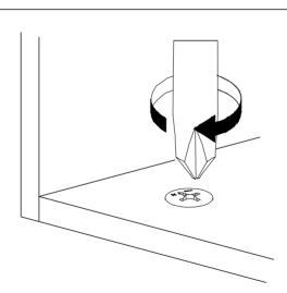
Turn cam lock clockwise to tighten.
