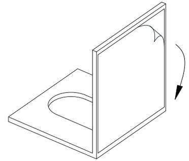
Peel the liner off of tape/
