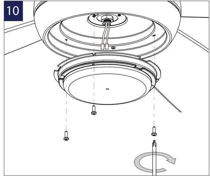
1. Remove 3 screws from outer perimeter of the adapter plate.
