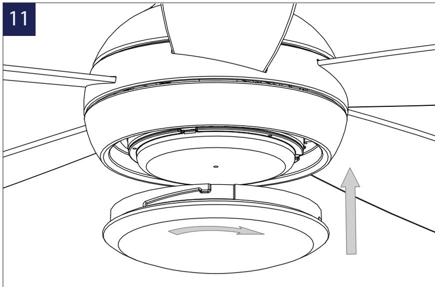
1. Install PC shade without over-tightening.
