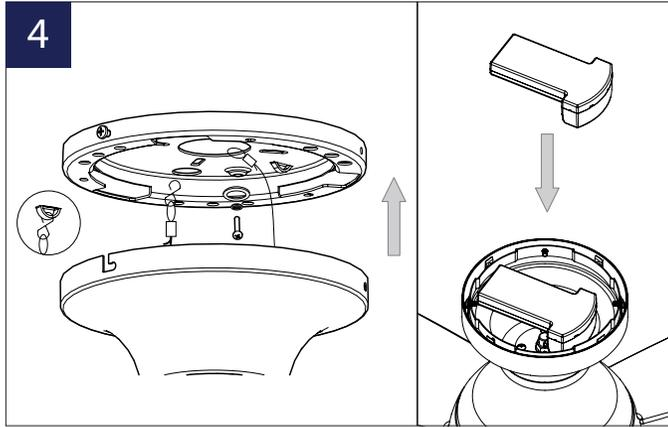
1. Remove 1 opposing screw and loosen the other 2 for the mounting bracket.
