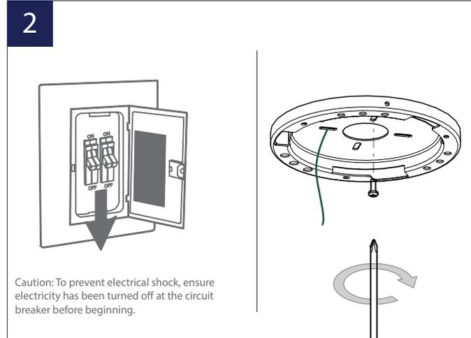
1. Attach the mounting bracket to the outlet box with two screws and washers provided. Make sure the bracket is tight and secured. For UL Junction box installation, use **A** parts.
