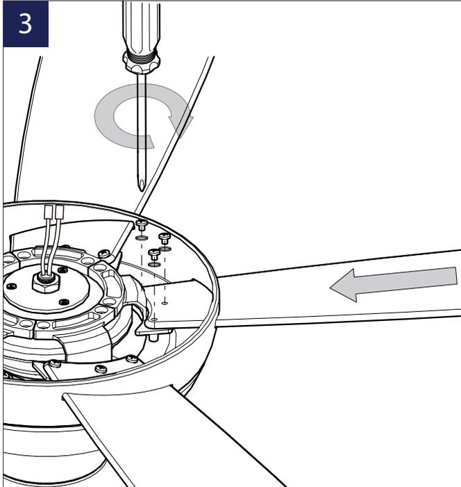
1. Insert blades in slots, aligning with motor assembly holes.
