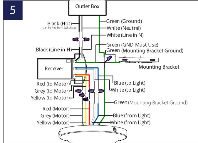
1. Connect the labeled wires from fan motor to the corresponding wires on the receiver.
