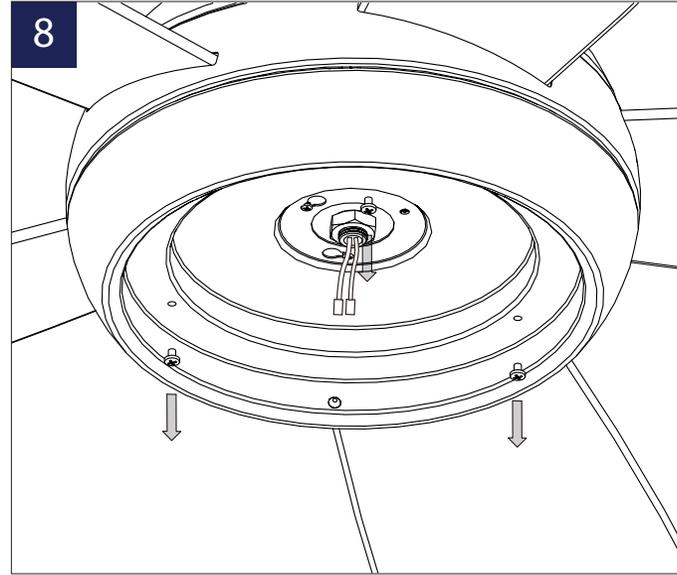
1. Remove 1 of 3 screws from the mounting ring and loosen the other two (do not remove).
