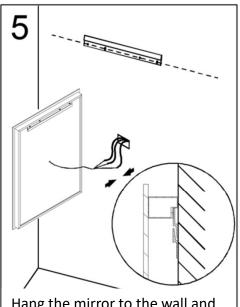
Hang the mirror to the wall and make sure the bracket in the back of the mirror lineup with the mounting bracket properly.
