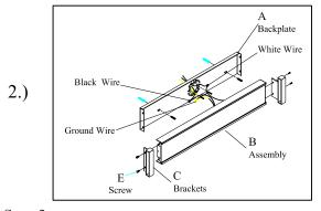
Step.2: Wire fixture to wires in outlet box. Copper wire is for Ground. Attach assembly (B) to the backplate (A) running screws (E) provided through the brackets (C) before tightening.
