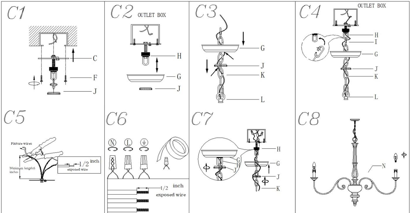
Step C1: Attach single bar (C) to outlet box with mounting screw (F). The side of single bar marked "GND" must face out.
