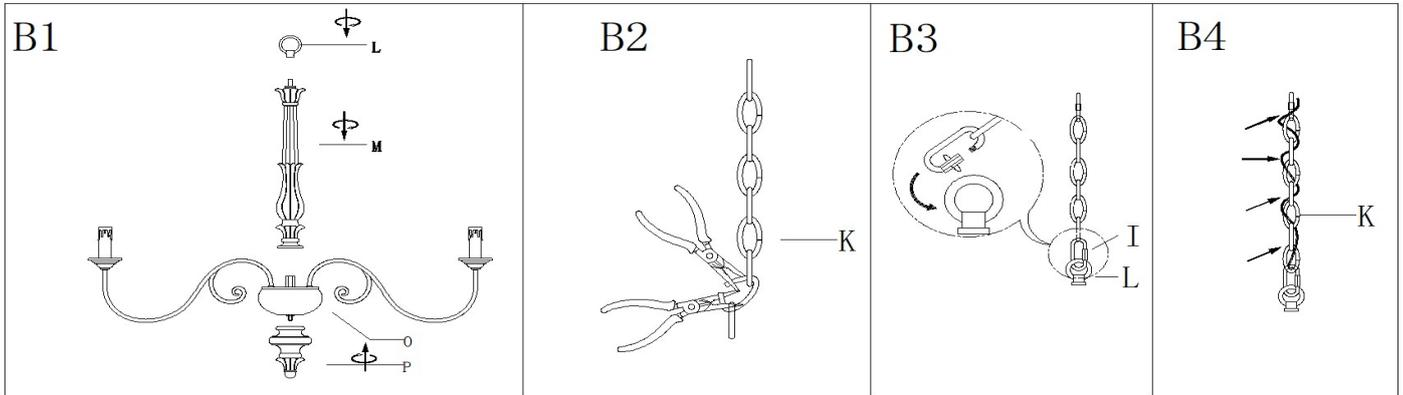
Step B1: Carefully thread post (M), drops (P) onto the fixture (O), then thread the loop (L) onto the post (M).
