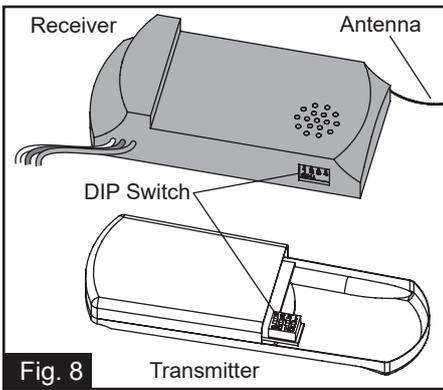
There is a code switch in the transmitter and receiver. This "DIP Switch" is a 4 key units (Fig.8). All keys were set at "ON" position in the beginning. Set the keys to a different code. Make sure the same numbered keys are switched "ON" for both DIP switches (Fig.8a). If the remote controlled fans are installed than one or the frequency is interfered, the fan may function abnormally.
