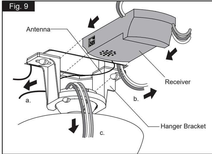
Move Ground Wires (a), Outlet Box wires (b), and Motor Wires (c) away from the center of the Hanger Bracket. Then slide Receiver through Hanger Bracket as shown, Antenna end first, until it is centered. Finally, cut Motor Wires (c) to length needed for connections.
