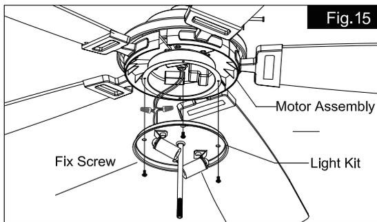
Connect the blue wire from motor to the black wire from light kit by wire connectors. And connect the white wire from motor to the white wire from light kit by wire connectors. Remove one fix screw from bottom of motor assembly (for later use), and loosen the other three fix screws. Secure the light kit to motor assembly with previous fix screw and tighten the other three fix screws.
