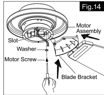
Rotate the motor to remove the motor screws and washers through a slot from the fan motor assembly. Secure blade brackets to the motor with washers and motor screws through a slot.
