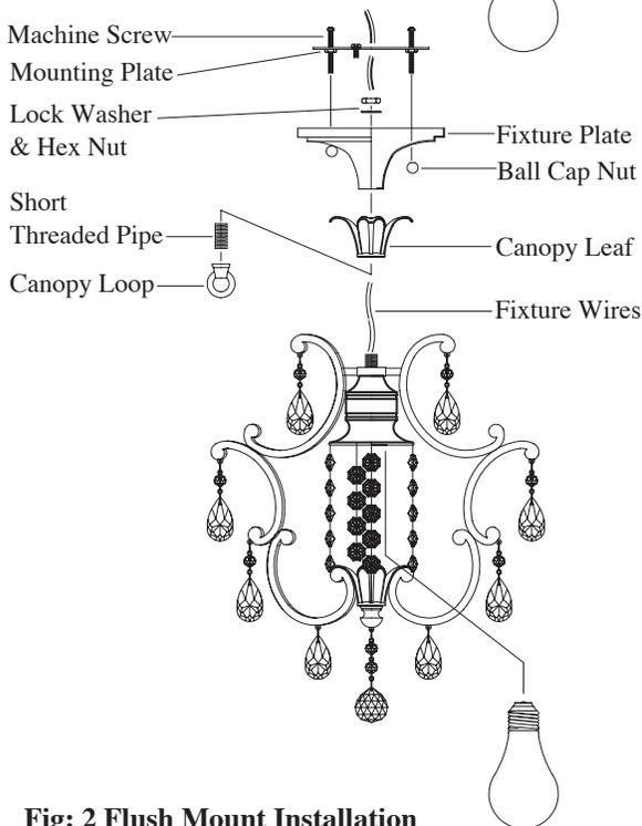
**Fig. 2 Flush Mount Installation**
