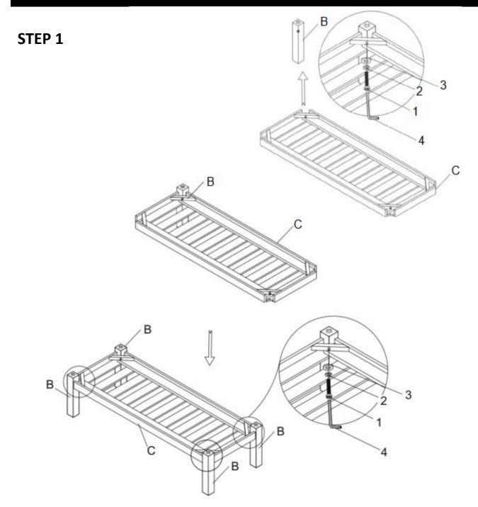
Attach Legs (B) to corners of Shelf (C) with Bolt (1), Lock Washer (2) and Flat Washer (3).
