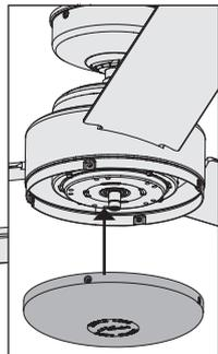
Lift the cap and align cap holes with the extend tabs of the fan housing.
