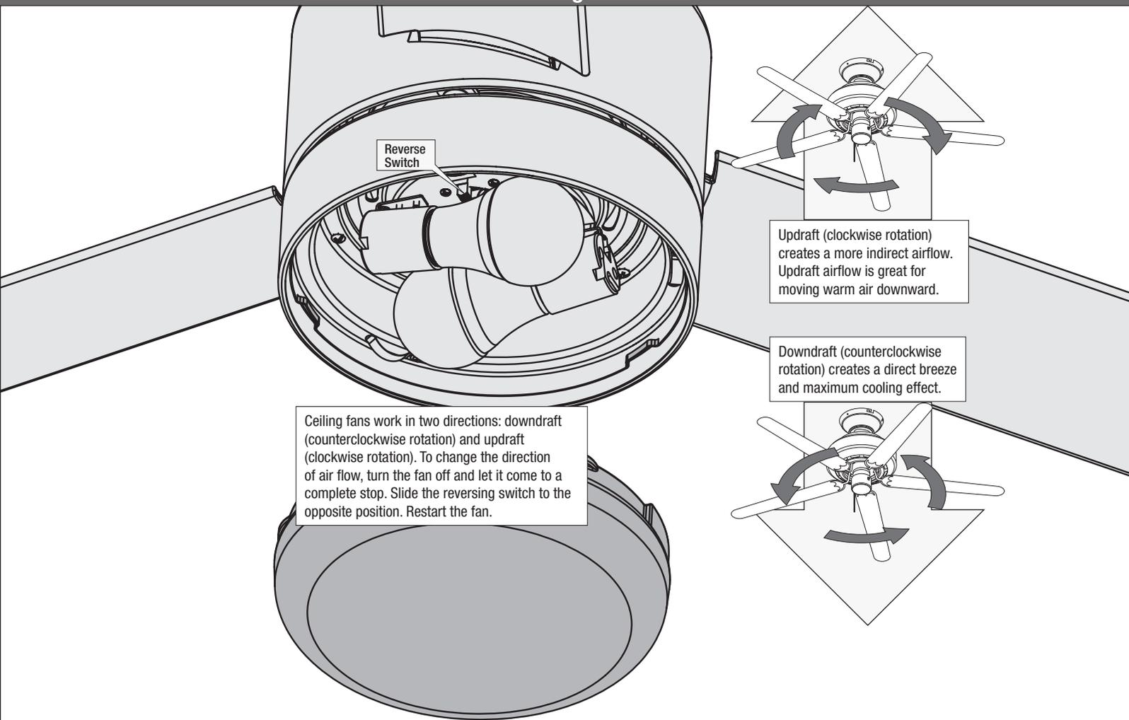
Ceiling fans work in two directions: downdraft (counterclockwise rotation) and updraft (clockwise rotation). To change the direction of air flow, turn the fan off and let it come to a complete stop. Slide the reversing switch to the opposite position. Restart the fan.
