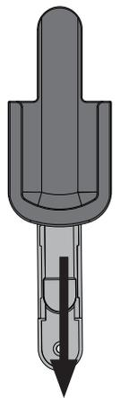
Slide the cradle onto the mounted bracket.
