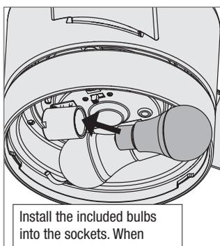
Install the included bulbs into the sockets. When necessary, replace with bulbs of same wattage.
