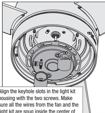
Align the keyhole slots in the light kit housing with the two screws. Make sure all the wires from the fan and the light kit are snug inside the center of the light kit, not pinched in between the upper switch housing and the light kit or hanging out of the sides.
