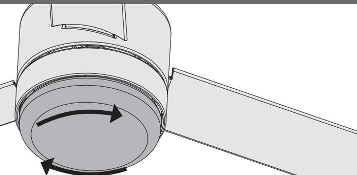
Attach the globe by lifting and turning clockwise one third of a full turn of the globe until it stops.
