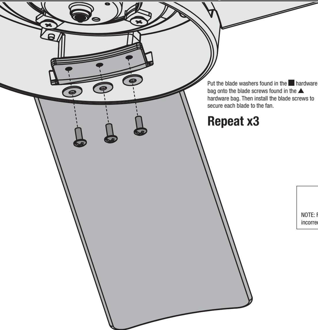
Put the blade washers found in the ■ hardware bag onto the blade screws found in the ▲ hardware bag. Then install the blade screws to secure each blade to the fan.
