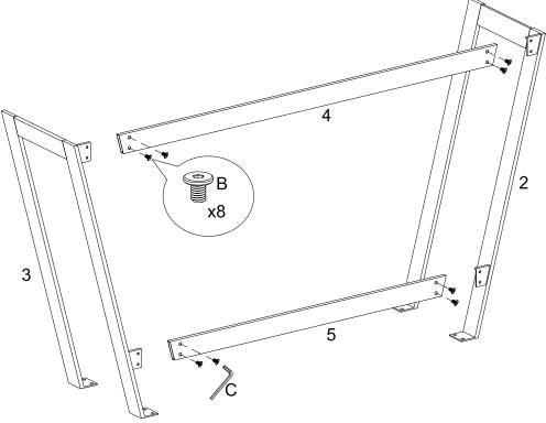
Attach part (4,5) to part (2,3) using bolt (B) with hex key (C).
