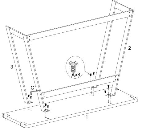
Attach part (2,3) to part (1) using bolt (A) with hex key (C).
