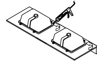
Apply sealant around the top edge of the sink rim. Flip top over and align basin to cutout. Screw in threaded bolts to each block. Secure plates with washer then wing nuts.
