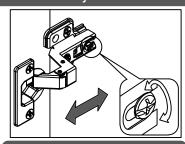
To adjust the depth, loosen up this screw, align, then retighten
