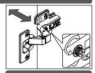
To adjust side-to-side, either loosen up or tighten this screw.
