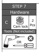
Use cam locks **C** to assemble the left side panel **6** to the main top panel **12**, and the partition panel **9** to the shelf **8** as shown.
