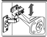
To adjust the height, loosen up these screws, align, then re-tighten
