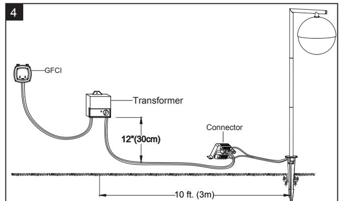
4. To insure uniform brightness the first fixture should be a minimum of 10 feet (3 meters) from the transformer (not included). (Fig.4)
