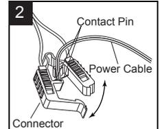
2. Open the connector from the fixture wires and insert the power cable from the transformer (not included) into the connector. (Fig.2)
