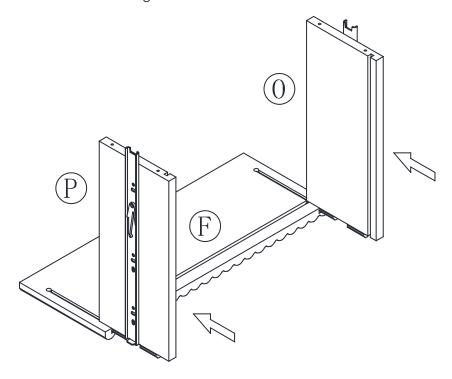
◆ Slide the DRAWER BOTTOM (K) into the grooves, in the DRWAER SIDES (O and P), and the DRAWER FRONT (F).
