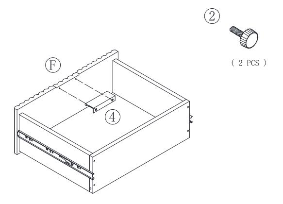
To insert the DRAWER into your unit, line up the EXTENSION SLIDES on the drawer with the EXTENSION RAILS on the unit and push the drawer into the unit until the drawer is fully inserted.
