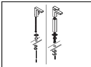
(2a) **For 1-Hole Installation:-** Install mounting bolt.
