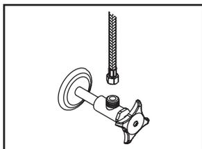
(3) Connect hot and cold inlet supply hoses to supply stops. For 1/2" connection; use 3/8" male to 1/2" female adapter for installation. Adapters are optional and not provided with the faucet.
