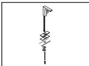
(2b) **For 3-Hole Installation:-** Install mounting bolt. Place deck plate with gasket under the faucet then place faucet in position on the sink. Slide mounting washer and mounting plate through mounting bolt from underneath of the sink, tighten locknut to mounting bolt.
