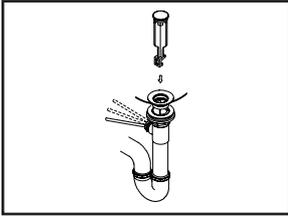
(6) Push pivot rod down, insert drain plug carefully. Test to ensure drain plug works properly.
