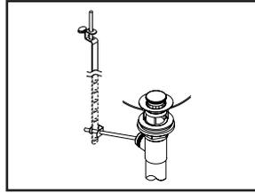
(7) Connect lift rod strap to pivot rod by using clip. Tighten the thumbscrew to connect lift rod strap to pop-up lift rod.
