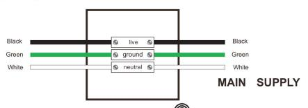
• After the product is connected to the circuit, the switch on the mirror surface will illuminate.
