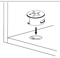
Quickfit head should be in the center of the cam lock. When the two panels are joined. Cam lock should be inserted before quickfit.
