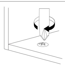
Turn cam lock clockwise to tighten.
