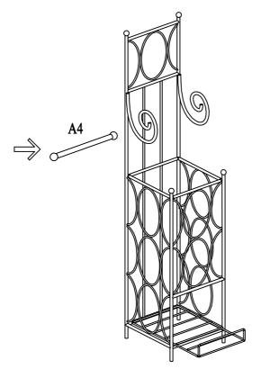
Attach Paper Bar (A4) to Top Frame (A2) as shown above.
