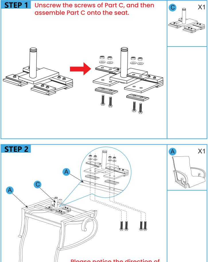
Please notice the direction of Part C and assemble it like the picture shows.
