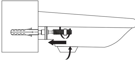
6. Ensure sink is secure, tighten bolts if necessary. Install faucet and drain using manufacturer's instructions. Connect to water supply and check for leaks.
