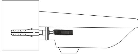
5. Screw metal nut onto each fixing bolt to secure the basin. Do not overtighten, as this may damage the ceramic.
