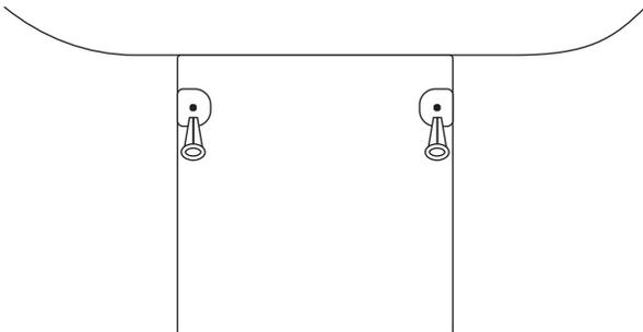
3. Slide shroud into place and secure using same steps as when mounting the sink. Use cover caps to hide hardware. Do not overtighten, it may crack the ceramic.
