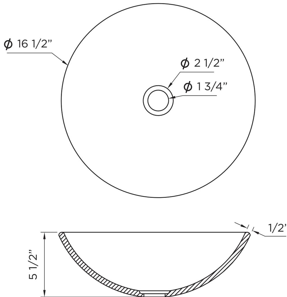
*ATTENTION! Dimensions may vary by up to 3/8". It is highly recommended to pull all dimensions of actual model for installation and measuring purposes.*
