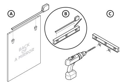
Press the anchors in the holes then insert screws with a drill or a screwdriver leaving just a tip outside of a wall.
