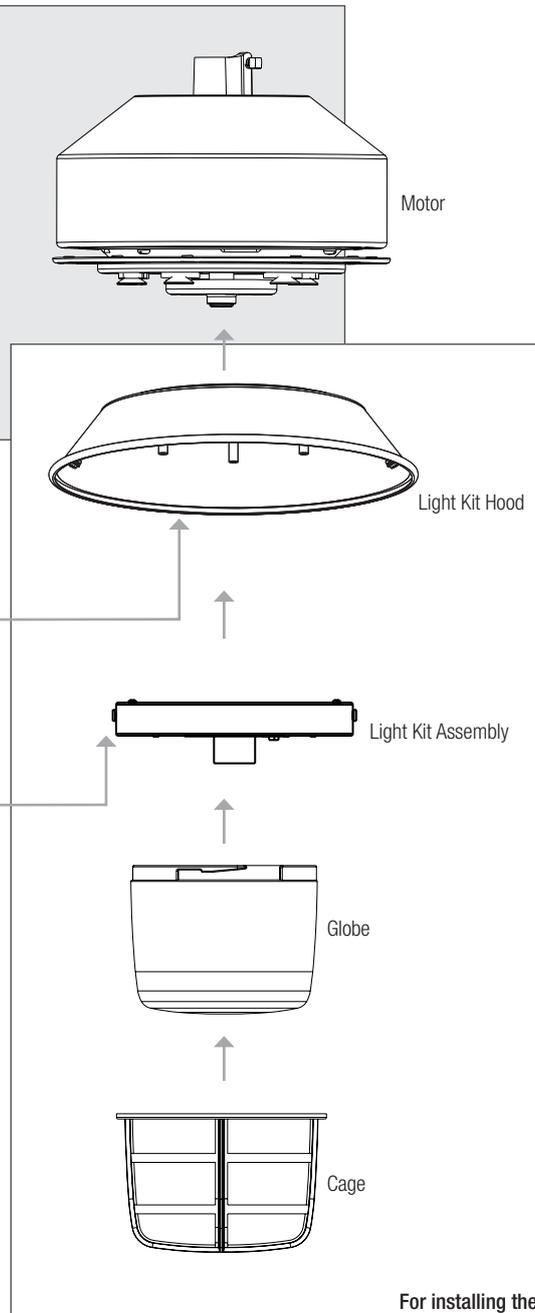
For installing the light fixture
