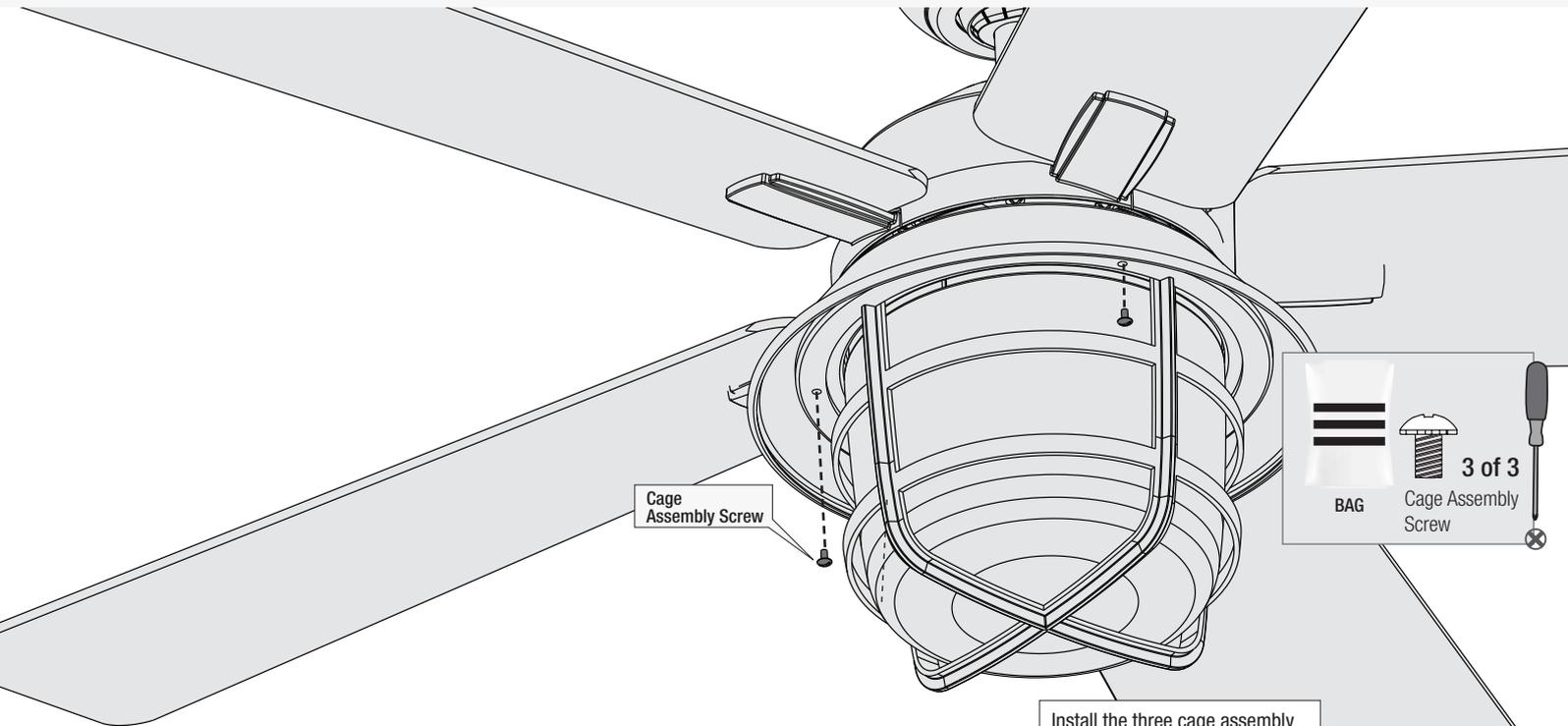
Install the three cage assembly screws and tighten all three screws securely.
