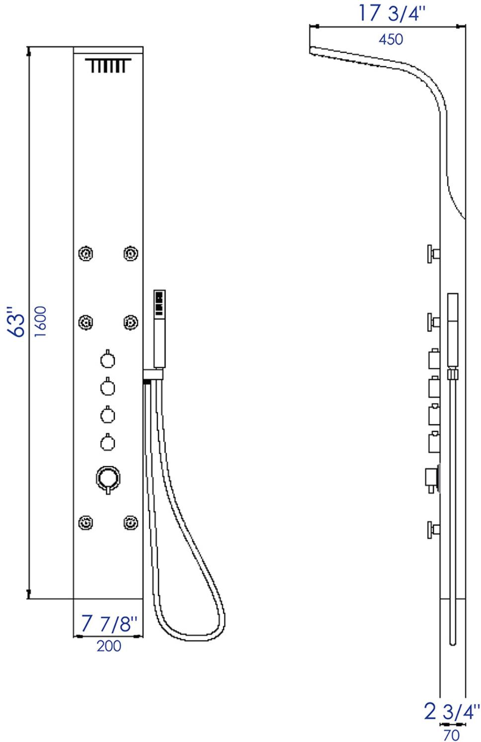
**Note:** All product dimensions are approximate and should be verified on site prior to installation.
